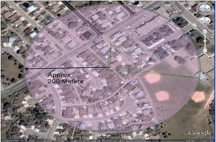
Figure 13 PlayStation 3 AP Potential Beacon Reception Area - Second Floor
